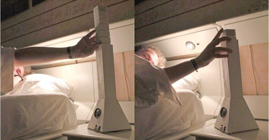
**Fig. 3.** The haptic peripheral alarm clock in context. Bedside lighting just for illumination of the evaluation setting.
